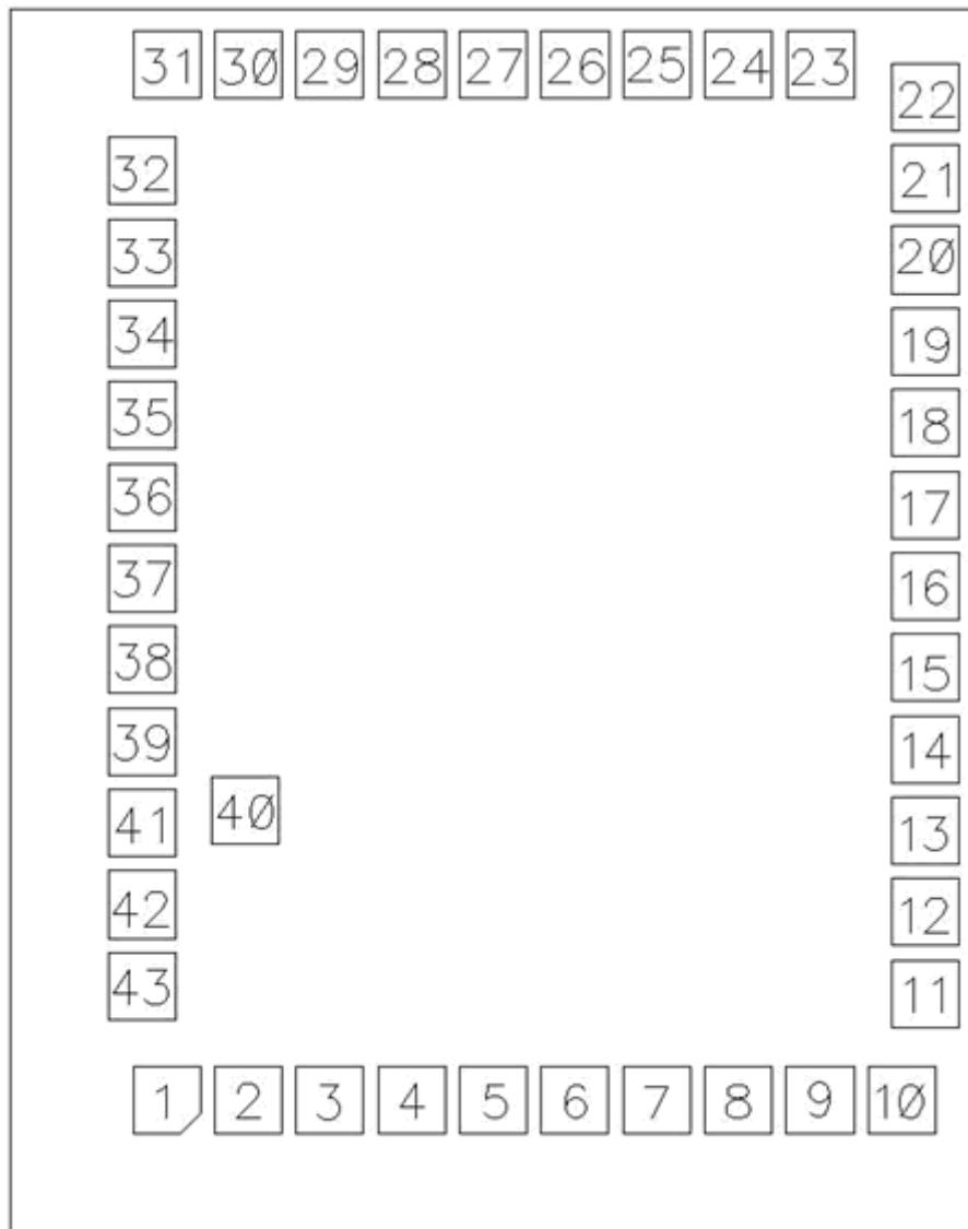
Substrate Size: 1500μm×1800μm
